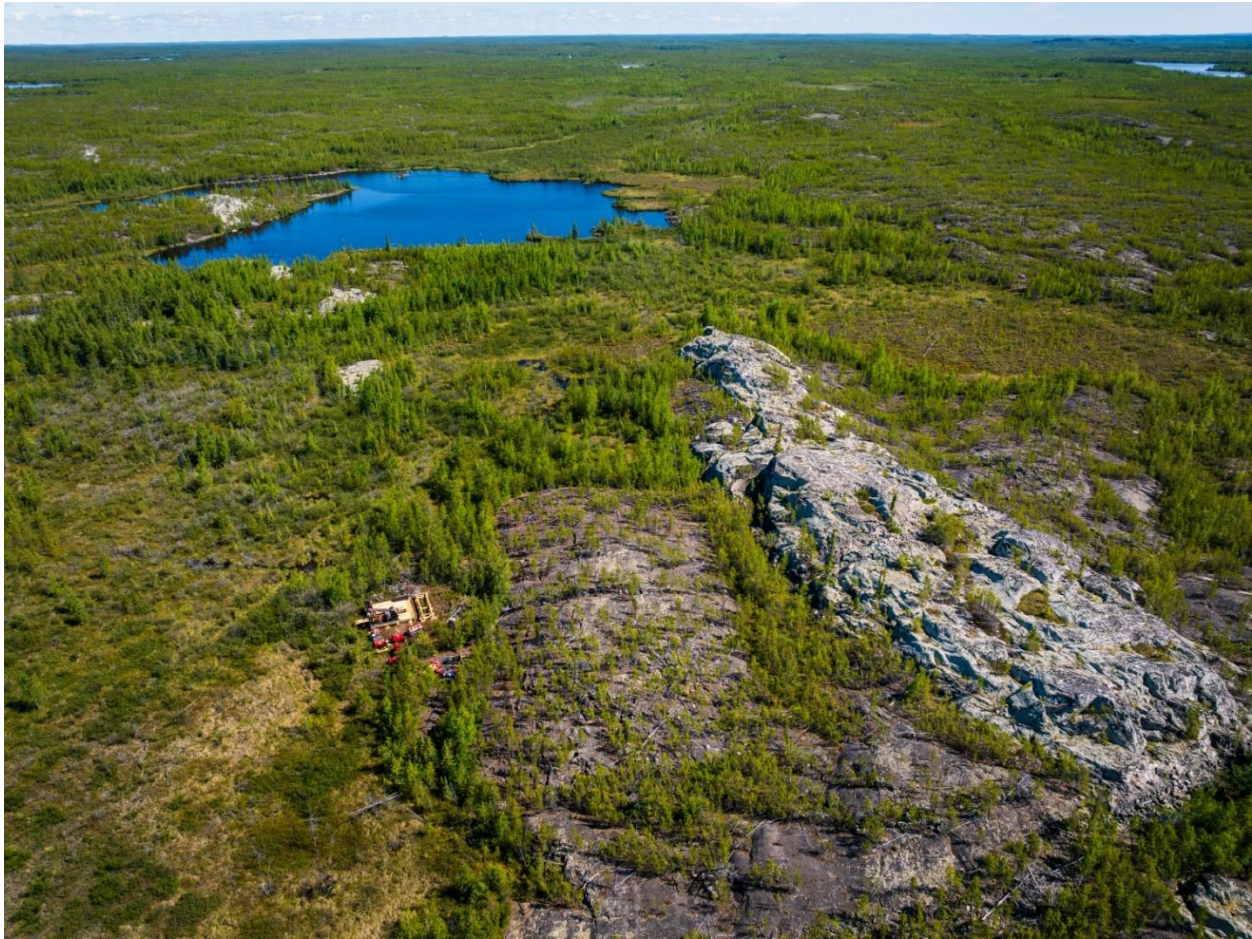
Large pegmatite outcrop (white) within Burwash Formation metasedimentary rocks. A diamond drill is stationed left of the pegmatite (Source: Li-FT, 2023).
