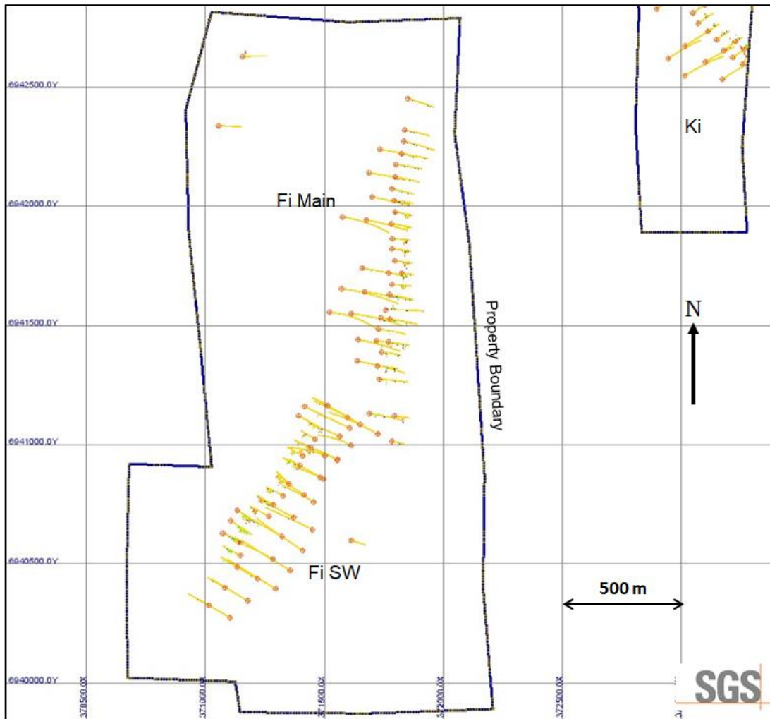
Figure 14-3 Plan View: Distribution of Surface Drill Holes in the Fi Main and Fi SW Deposit Areas
