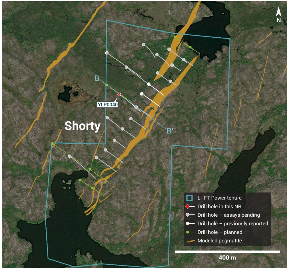
Figure 4 – Plan view showing the surface expression of the Shorty pegmatite with diamond drill holes reported in this press release.
