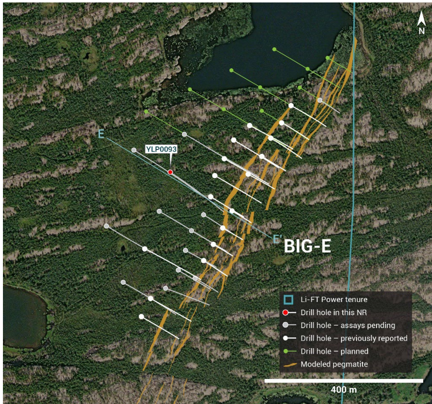
Figure 2 – Plan view showing the surface expression of the BIG-East pegmatite with diamond drill holes reported in this press release.
