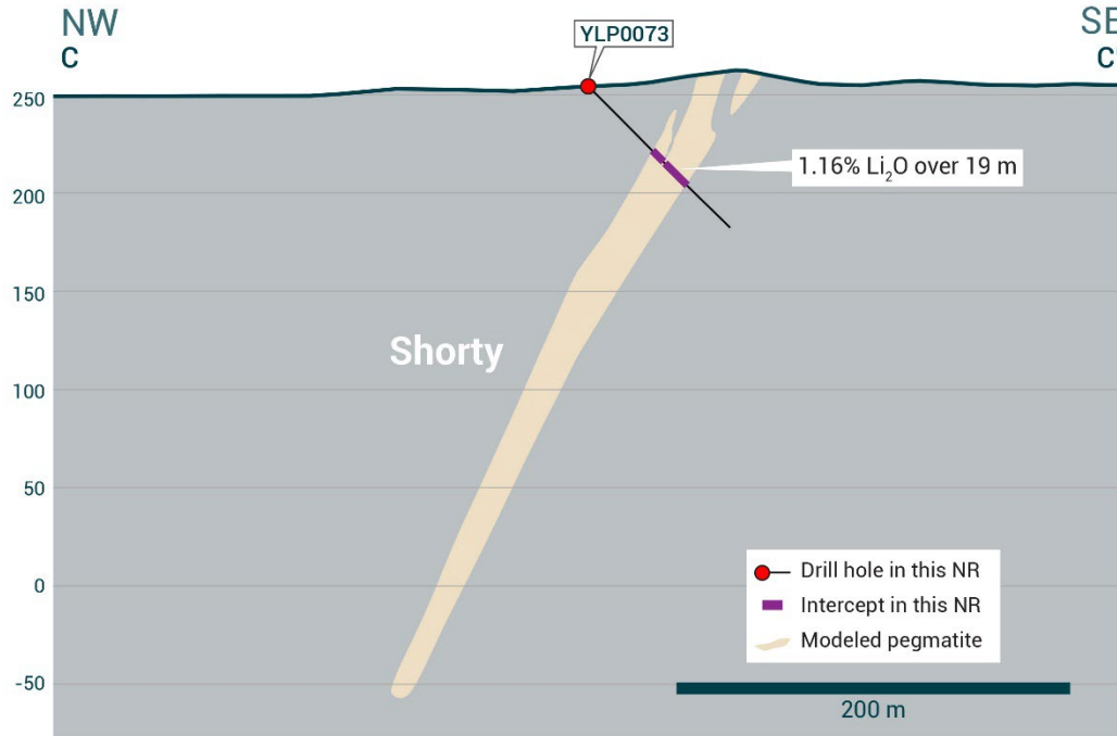
Figure 5 – Cross-section illustrating YLP-0073 with results as shown in the Shorty pegmatite dyke with a 19 m interval of 1.16% Li 2 O.
