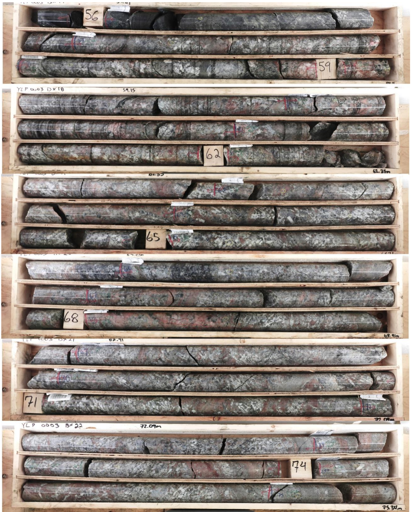
Figure 4a – Core photos of drill hole YLP0003. Spodumene-bearing pegmatite was intersected from 55 to 94 meters (intersect continues on next page).
