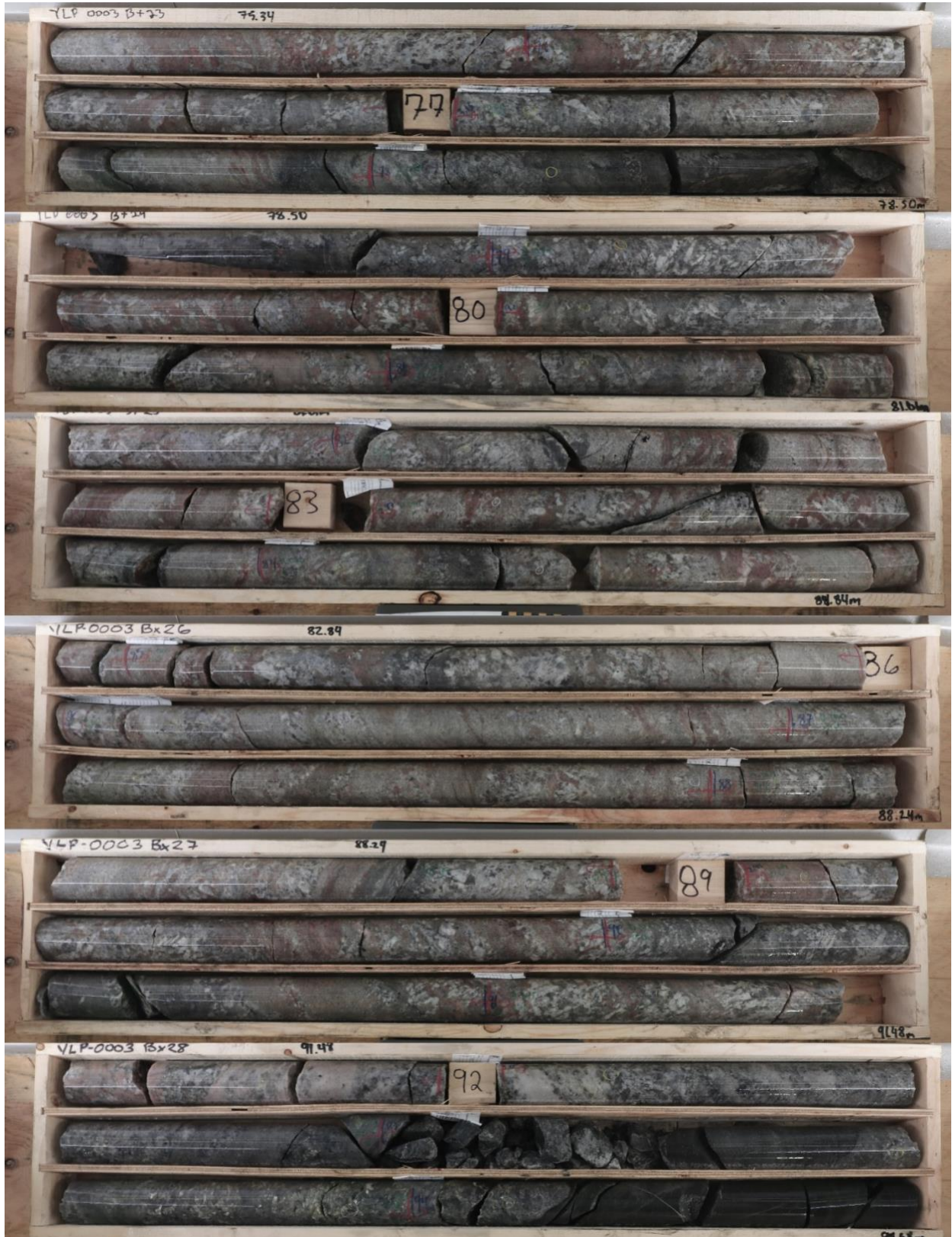
Figure 4b – Core photos of drill hole YLP0003. Spodumene-bearing pegmatite was intersected from 55 to 94 meters.
